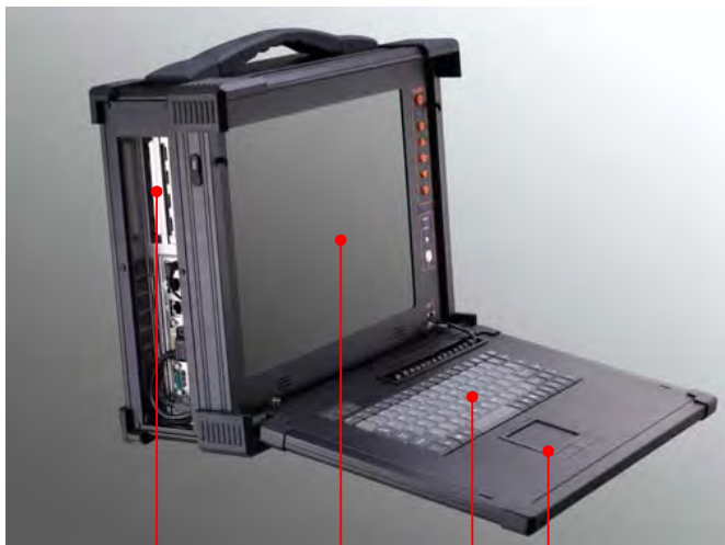
2×Full-Size Expansion Slots 15" TFT LCD Touchpad 88 keys keyboard
