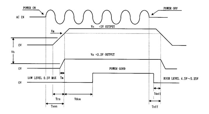
Vn Nominal voltages +5V Vm Minimum voltages +4.5V Nominal voltages +3.3V Va Vb +2.0V max Tson Switch on time (500 ms. max.) Trs +5V rise time (50ms. max.) Tdon Delay turn-on (100ms. < Tdon < 500ms.) **Tdoff** Delay turn-off (1 ms. min.) Toff Hold up time (16ms Min)
