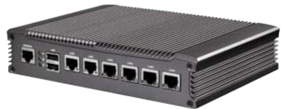
The Front Side of the LEC-2026: featuring 6 LAN ports, 2 USB and a COM port.
