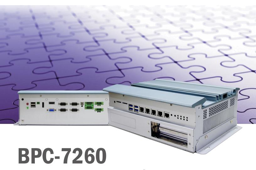
Fanless Embedded Box PC with 4th/5th Generation Intel® Core™ i Processor and PCI/PCIe Expansion
