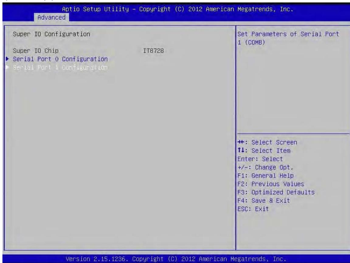
**Serial Port 0 Configuration:** Set Parameters of Serial Port 0 (COMB).
